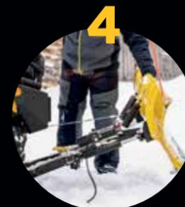
4 Remove the winch cable from the guide. You're ready to plow.
