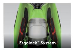
A narrow seat profile with deep knee pockets lets riders sit naturally and use the leg muscles to hold onto the machine for more control.
