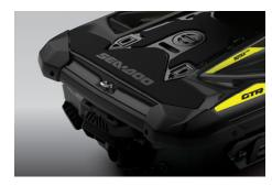
Exclusive quick-attach system on a large swim platform that allows for easy installation of storage accessories.
