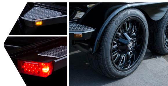
Key features include diamond plate step pads, a swing-away tongue for easy storage, and LED submersible lighting. (swing-away tongue N/A on 165 models).
